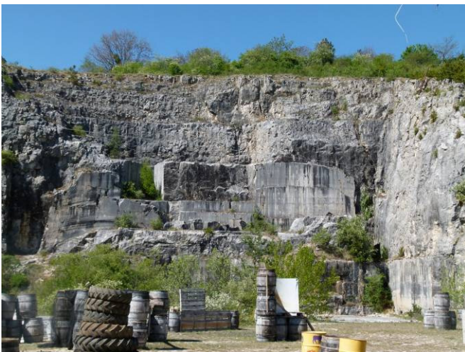
Valerôts quarry now inactive. The smooth sawn vertical faces are in the marble-producing Calcaire de Comblanchien Formation of the Middle Jurassic.
